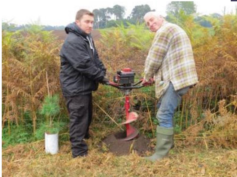
A mechanical auger being used to dig the holes for the new pine lines on Euston estate
